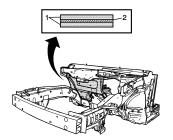
This information provides repair recommendations and general guidelines for steel classified as Laminated Steel. This type of steel is constructed by bonding 2 pieces of cold rolled steel (1) with a viscoelastic layer of adhesive (2).
